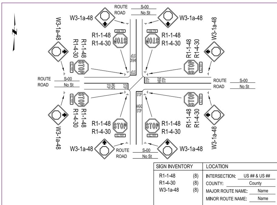
Figure 2. SCDOT's Template for Four-Way, Stop Controlled Intersections
