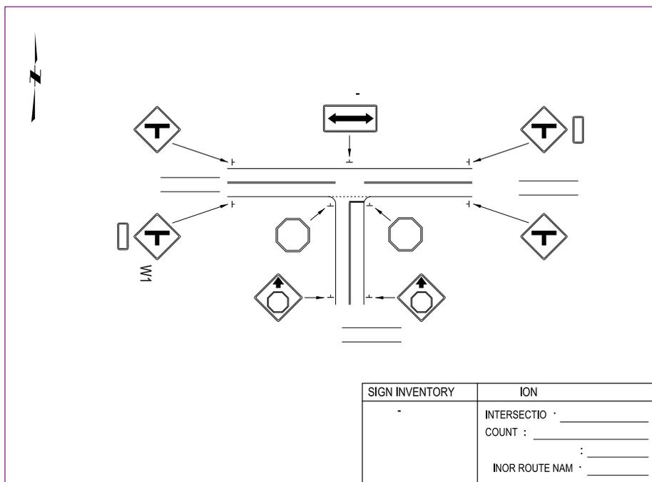
Figure 4. SCDOT's Template for T-Type, Stop Controlled Intersections
