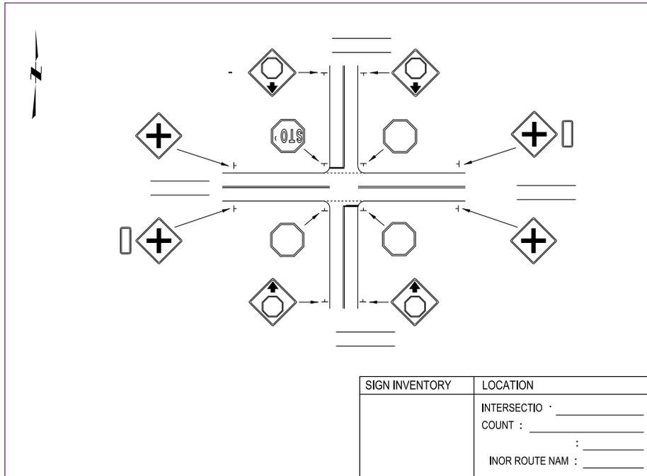
Figure 3. SCDOT's Template for Two-Way, Stop Controlled Intersections
