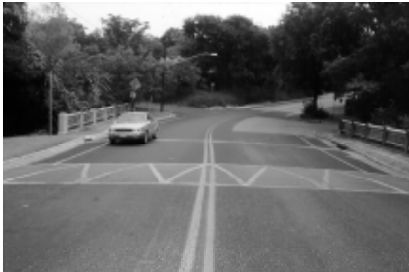
Figure 3.10. Speed Hump. (Austin, TX)
