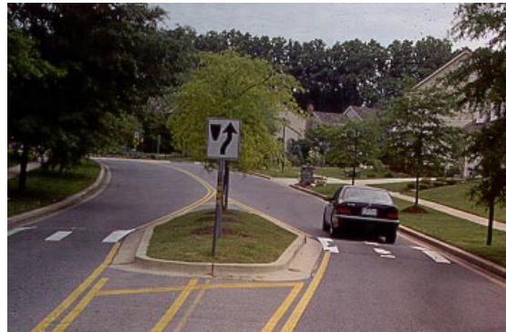
Center Island with Humps. (Montgomery County, MD)
