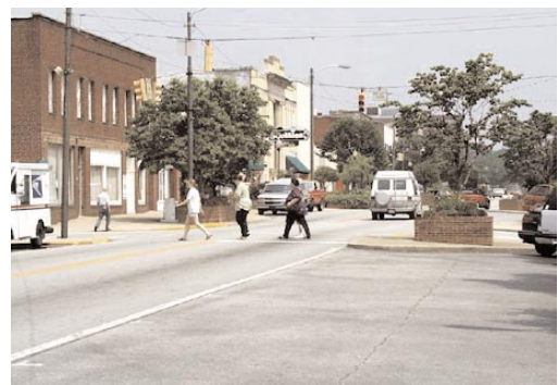
Bulb-outs shorten pedestrian crossing distance and slow down cars.
