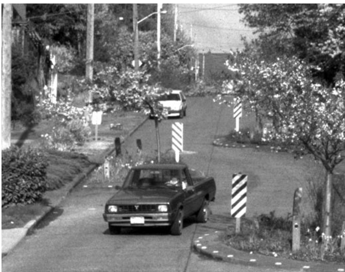
The chicanes pictured above narrow this residential street to one lane and require traffic to move slowly.
