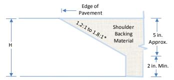
Note 1: The range of slope is equal to 29° to 40°.
