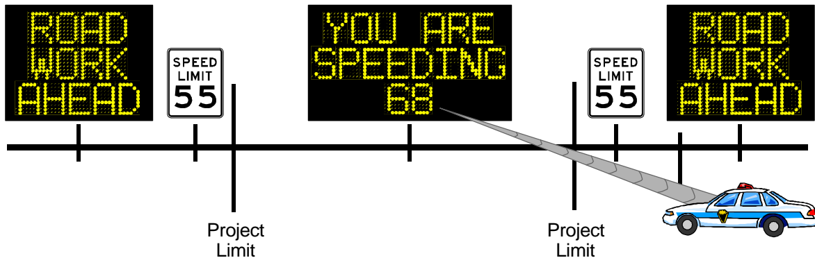
Figure X-53. Simplified Diagram of Positioning of Devices in Remote Enforcement.
