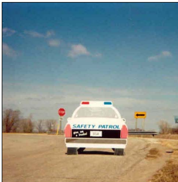
(a) Cutout car positioned on shoulder.
