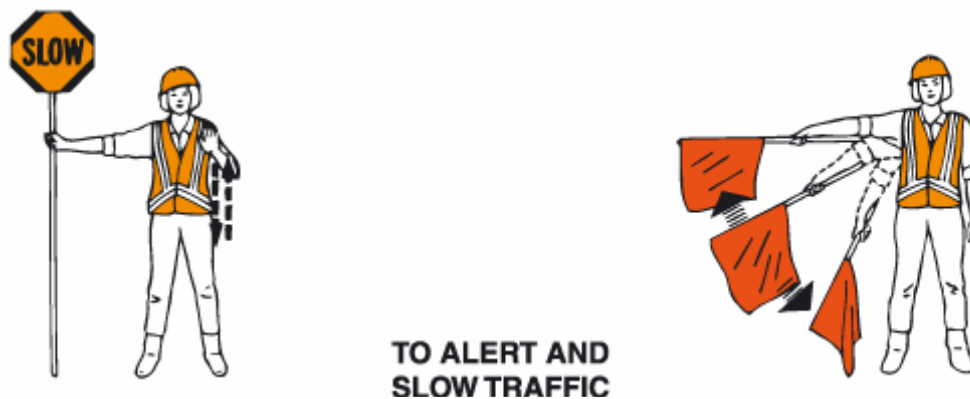
Figure X-42. TMUTCD "Alert and Slow" Flagging Method.
