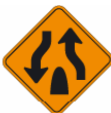
Figure X-27. Divided Highway Ends Sign (CW6-2).
