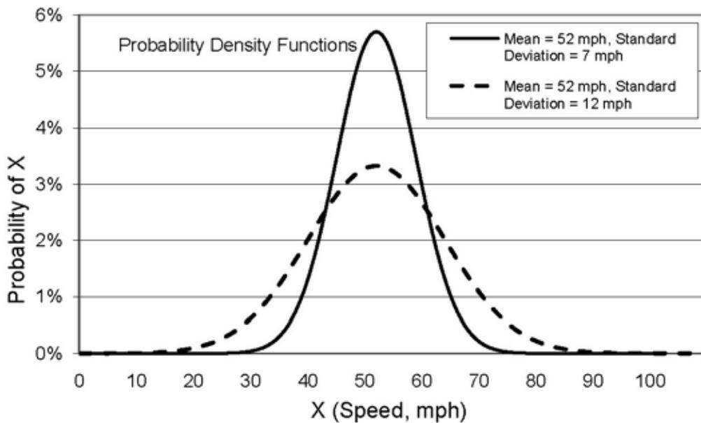
**Figure 7. Examples of two normal probability distributions, operating speeds, same mean, different standard deviations.**
