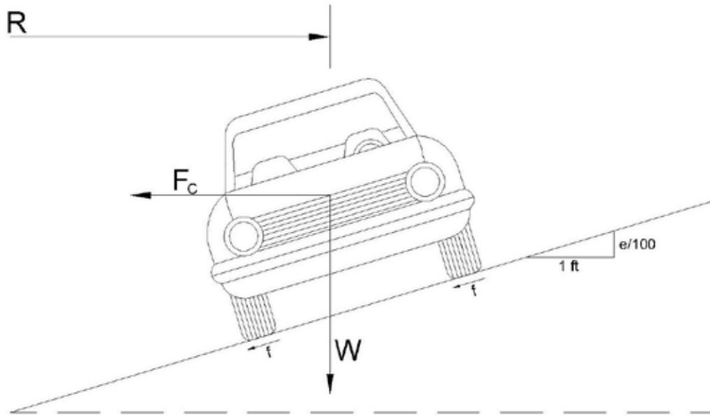
**Figure 4. Cross section of vehicle on superelevated road.**
