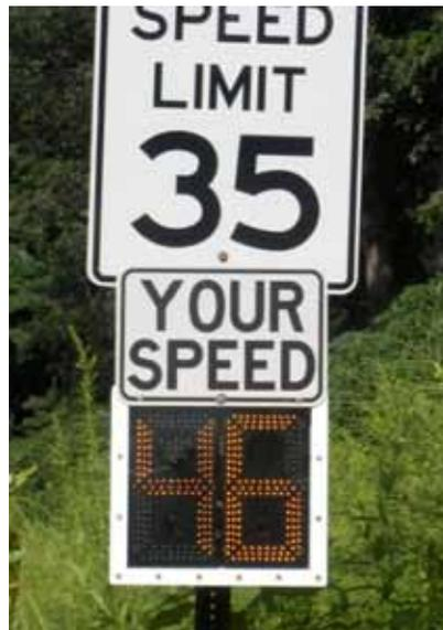
**Figure 21. Example dynamic speed display sign.**
