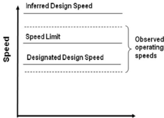
**Figure 17. Relationships that can result when speed limit is increased on basis of actual operation speeds.**
