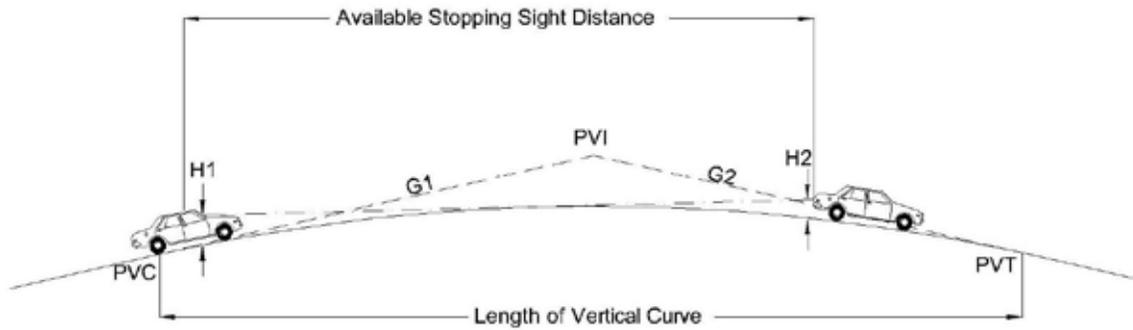
**Figure 2. Effect of crest vertical curves on sight distance.**
