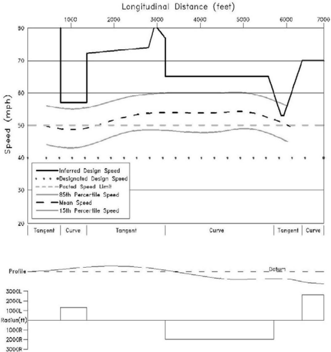
**Figure 11. Speed profile with inferred design speed substantially exceeding designated design speed.**
