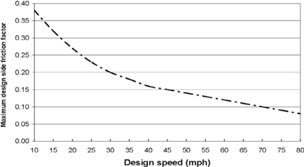
Figure 5. Maximum side friction factors for various design speed. Source: Ref (1)
