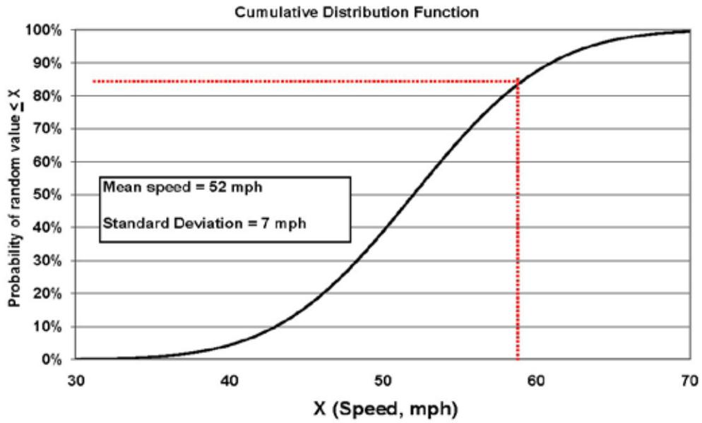
Figure 8. Example cumulative distribution function, operating speeds.
