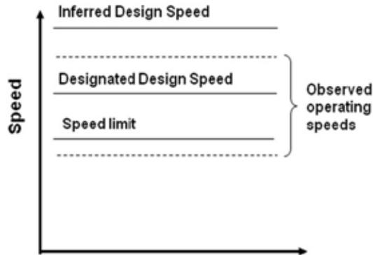
**Figure 16. Speed relationships that sometimes develop on low and moderate design speeds.**
