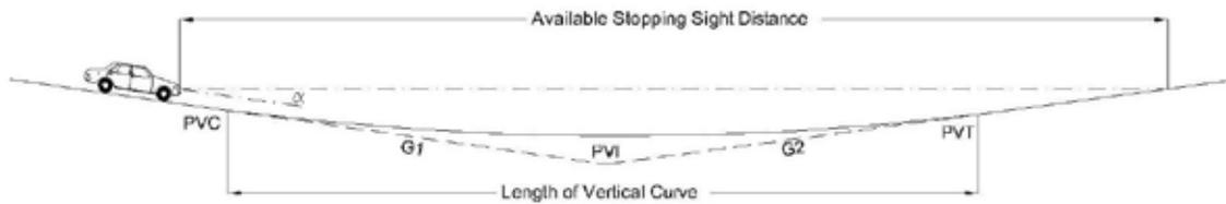
**Figure 3. Effect of sag vertical curves on sight distance.**
