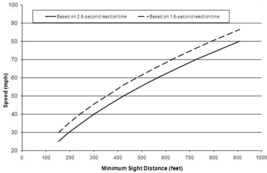
**Figure 10. Sight distances corresponding to different reaction times.**
