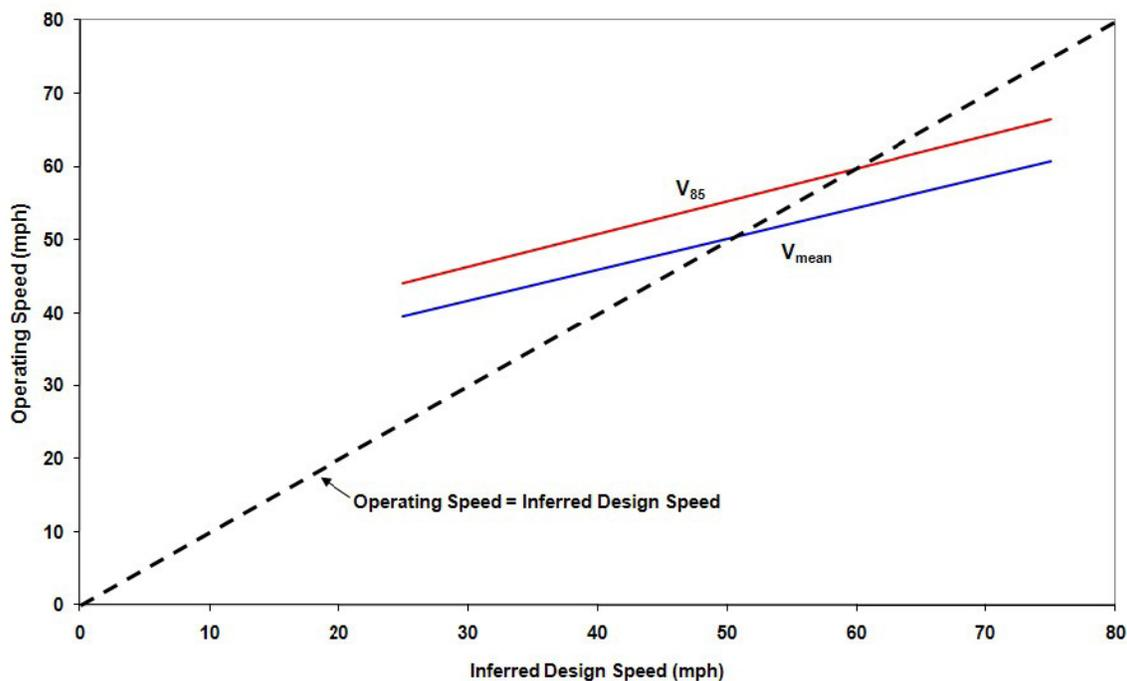
**Figure 18. Mean and 85<sup>th</sup> percentile speeds versus inferred design speed on horizontal curves.**
