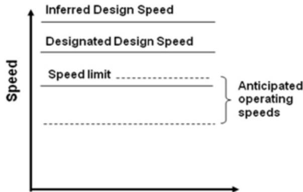
**Figure 15. Typical speed relationships contemplated by design process.**
