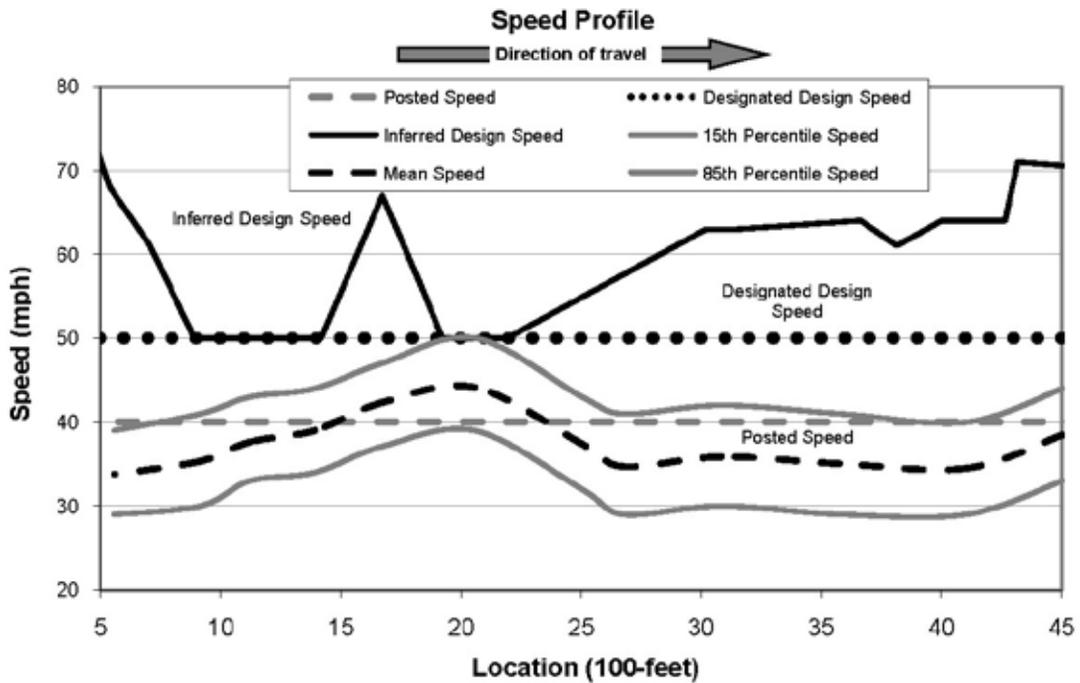
Figure 9. Example speed profile.
