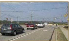
Coordination of traffic signals is one of the most cost effective ways of improving traffic flow along a corridor. Signal coordination involves operating the traffic signals, so that groups of vehicles can travel through the series of signals with minimal stopping.
