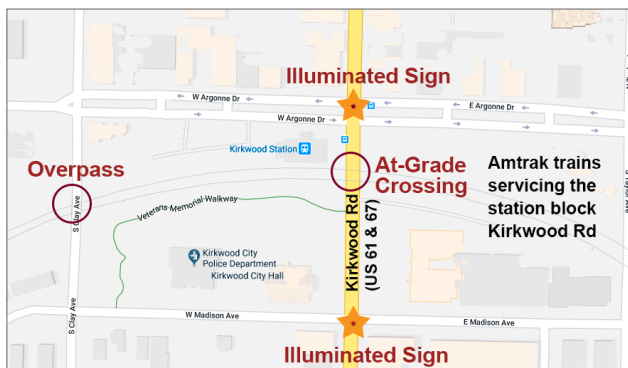
Locations of illuminated signs in advance of the Kirkwood Road at-grade crossing and the nearby overpass. Original map ©Google 2018.
