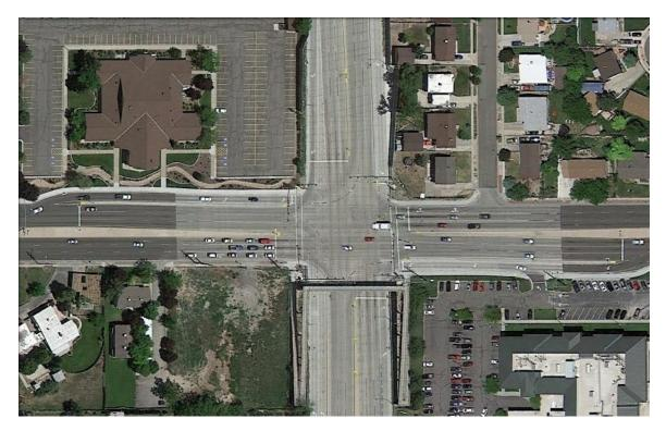
Exhibit 1-3. Four-legged DLT intersection with four displaced lefts (West Valley City, UT). $^{(1)}$
