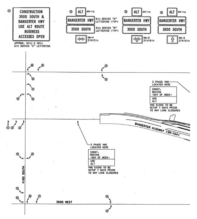
Exhibit D-3. Illustration. Detour routes for construction of DLT intersection in Salt Lake City, UT—south end.
