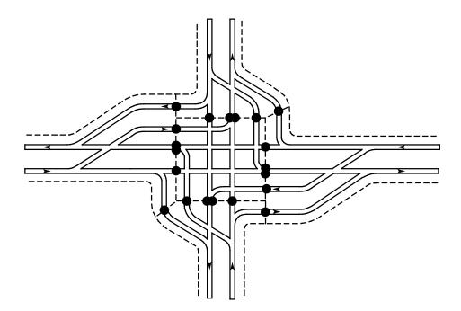
Exhibit 3-6. Pedestrian-vehicle conflict point diagram for a DLT intersection with four displaced left turns with a single-stage crossing.
