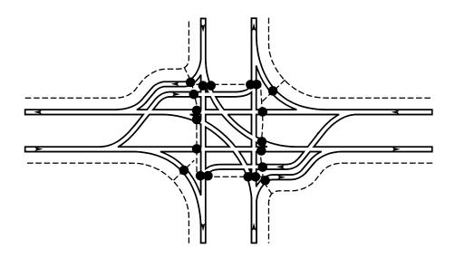
Exhibit 3-5. Pedestrian-vehicle conflict point diagram for a DLT intersection with two displaced left turns with a single-stage crossing.
