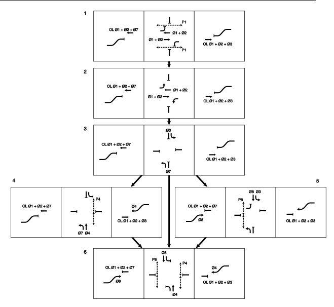
Exhibit 5-5. Signal phasing for a DLT intersection with major street displaced left turns with a single phase crossing for pedestrians.
