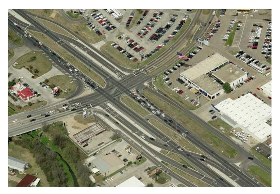
Exhibit 7-8. Four-legged DLT intersection with major street displaced left turns and channelized right turns (Baton Rouge, LA).<sup>(1)</sup>
