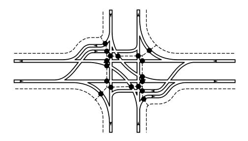
Exhibit 3-7. Pedestrian-vehicle conflict point diagram for a DLT intersection with two displaced left turns with a two-stage crossing.
