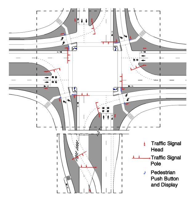
Exhibit 8-1. Possible signal pole and mast arm locations for a DLT intersection.
