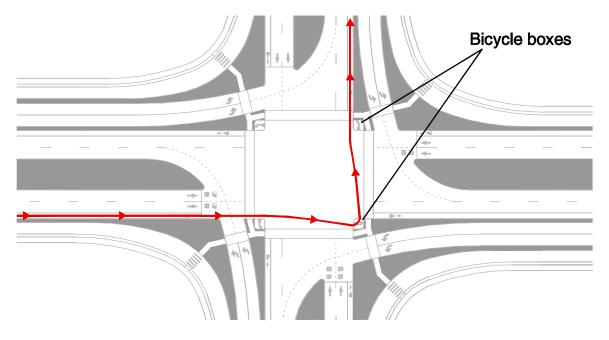
Exhibit 3-12. Accommodating on-street left-turning bicycles with a bicycle box through a DLT intersection.
