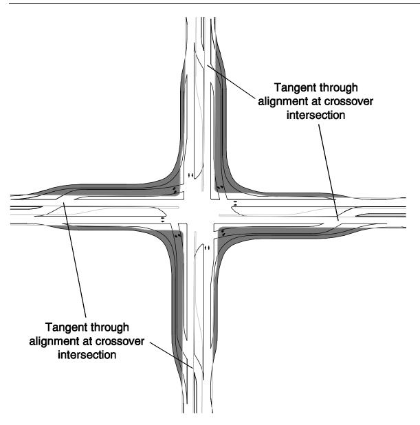
Exhibit 7-12. Footprint comparison of a DLT intersection with tangent through alignments versus a conventional intersection.
