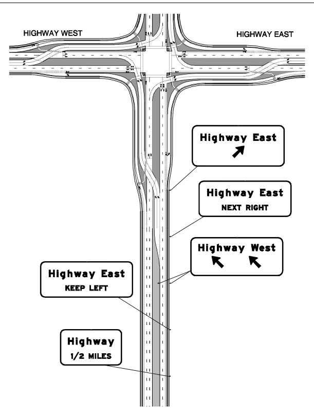
Exhibit 8-6. Example guide signing along an intersection approach for a DLT intersection.
