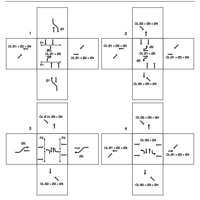
Exhibit 5-4. Signal phasing for a DLT intersection with a single controller.
