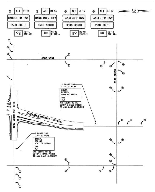
Exhibit D-2. Illustration. Detour routes for construction of a DLT intersection in Salt Lake City, UT—north end.
