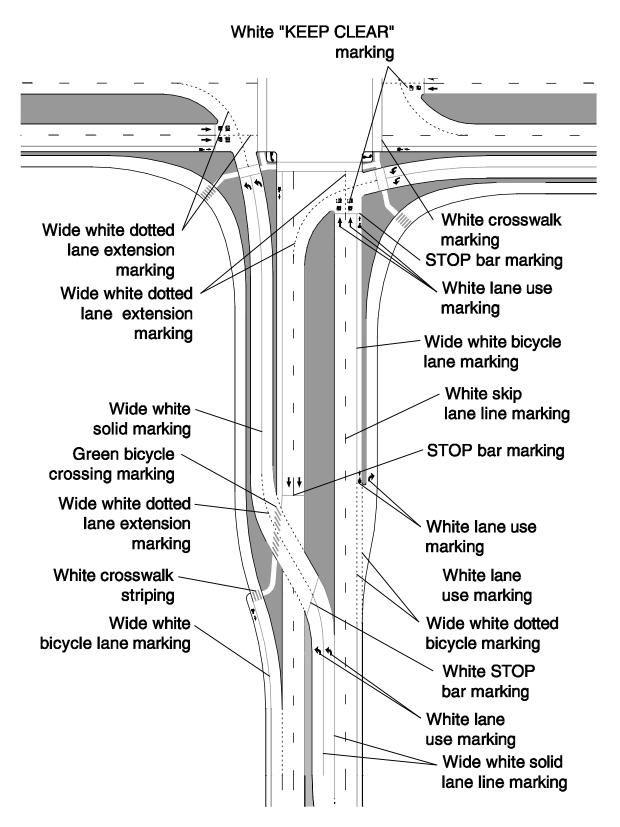
Exhibit 8-9. Pavement markings along an intersection approach for a DLT intersection.
