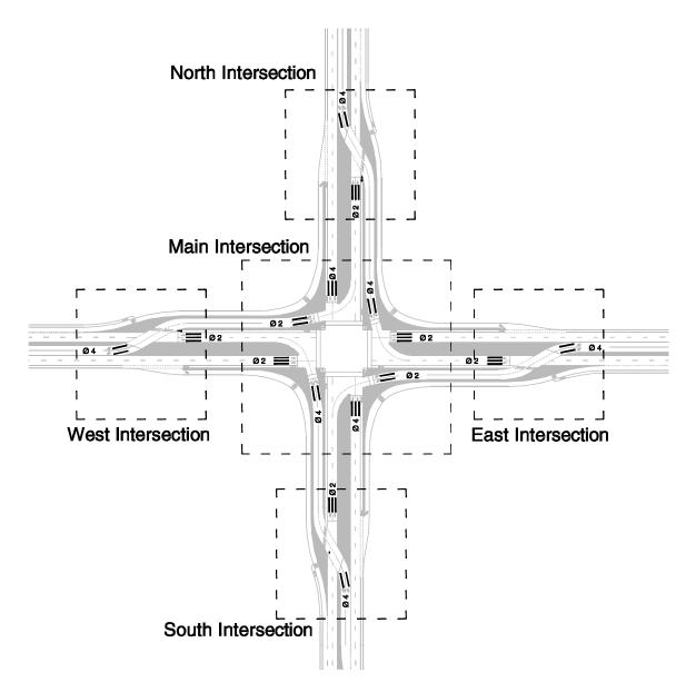
Exhibit 8-2. Possible detector placement locations for a DLT intersection with five separate controllers.
