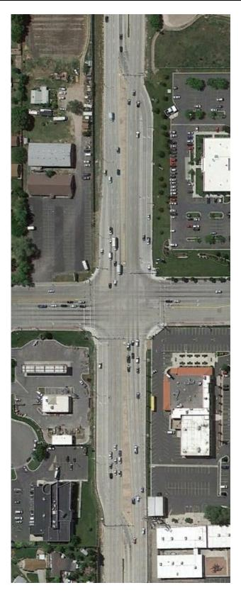
Exhibit 7-7. Four-legged DLT intersection with major street displaced left turns and without channelized right turns (West Valley City, UT).<sup>(1)</sup>
