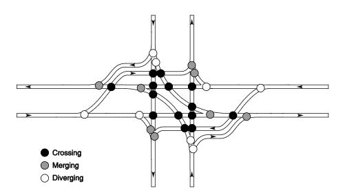
Exhibit 4-3. Conflict point diagram for a DLT intersection with two displaced left turns.
