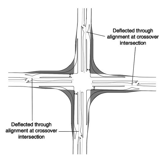
Exhibit 2-3. Footprint comparison of a DLT intersection with deflected through alignments versus a conventional intersection.
