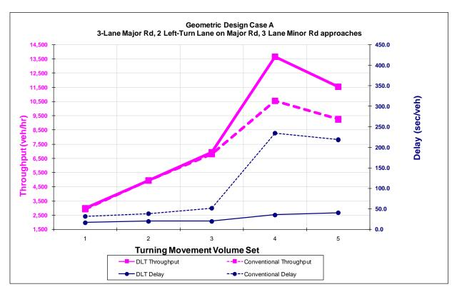
Exhibit B-3. Graph. Throughput and delay comparisons for geometric design case A—full DLT intersection.
