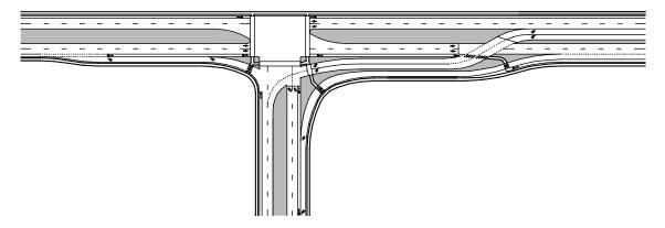
Exhibit 1-13. Three-legged DLT intersection with displaced left turns on major road approach.
