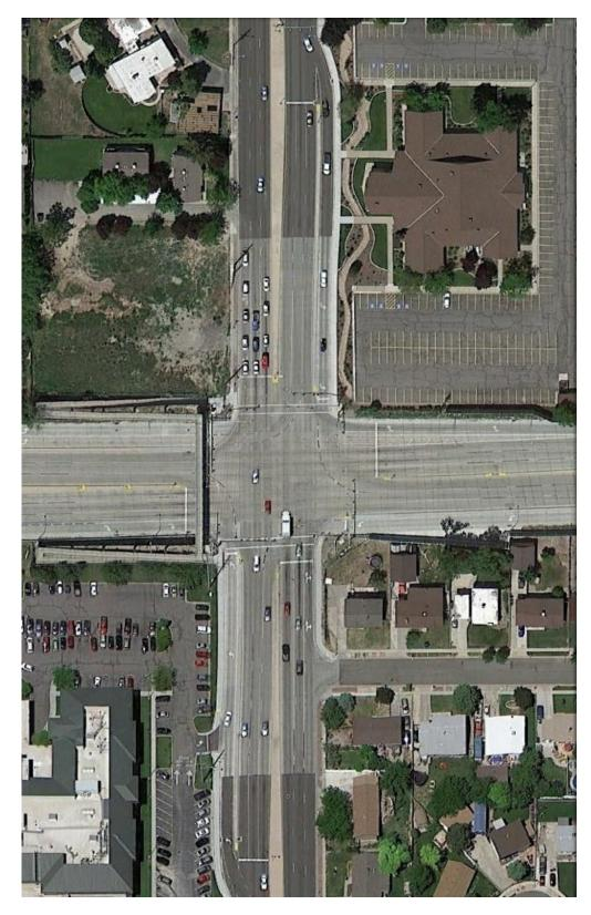
Exhibit 7-6. Four-legged DLT intersection with four displaced left turns and without channelized right turns (West Valley City, UT).<sup>(1)</sup>
