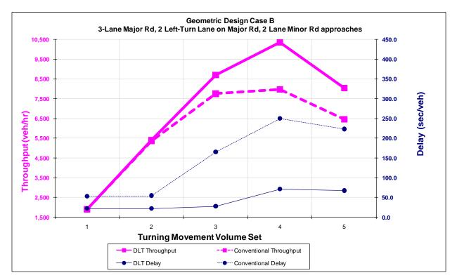
Exhibit B-5. Graph. Throughput and delay comparisons for geometric design case B—full DLT intersection.
