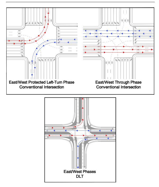
Exhibit 5-1. Concurrent movements for east-west arterial at conventional intersection and DLT intersection.
