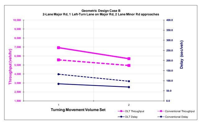
Exhibit B-6. Graph. Throughput and delay comparisons for partial DLT intersection geometric design case B.
