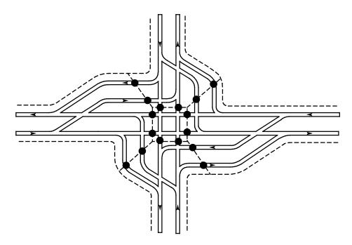
Exhibit 3-8. Pedestrian-vehicle conflict point diagram for a DLT intersection with four displaced left turns with a two-stage crossing.
