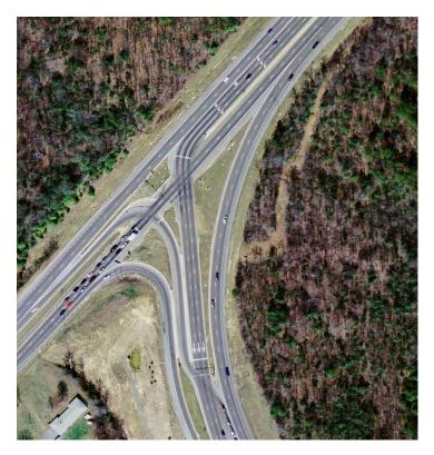
Exhibit 7-10. Three-legged DLT intersection with minor street displaced left turn (Accokeek, MD).<sup>(1)</sup>
