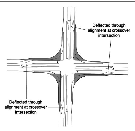
Exhibit 7-13. Footprint comparison of a DLT intersection with deflected through alignments versus a conventional intersection.
