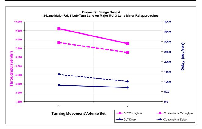
Exhibit B-4. Graph. Throughput and delay comparisons for partial DLT intersection geometric design case A.
