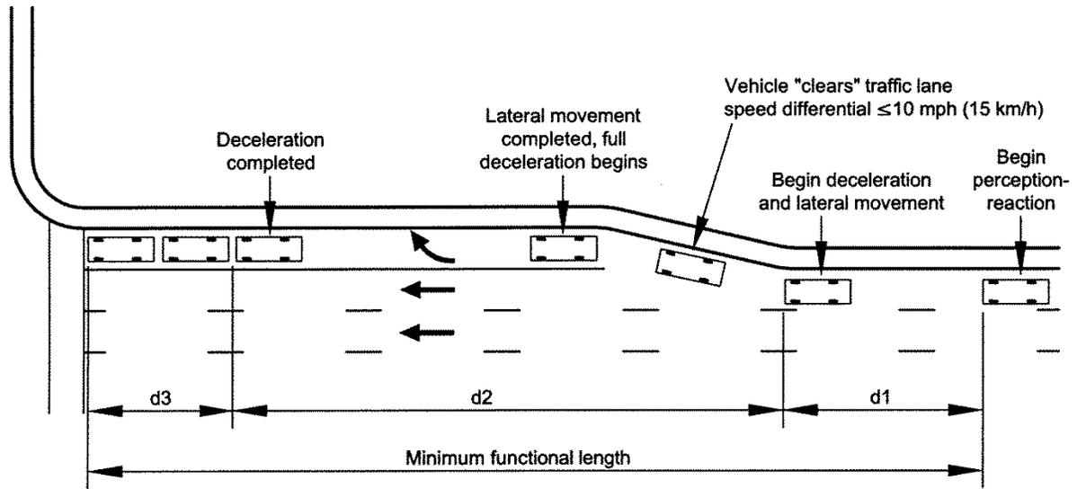
Exhibit 8-8. Diagram of the upstream functional area of an intersection.<sup>(90)</sup>
