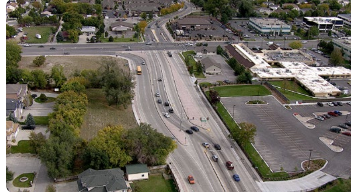
DLT Intersection at 6200 South and Redwood Road Source: DLT Case Study Video FHWA-SA-14-057
