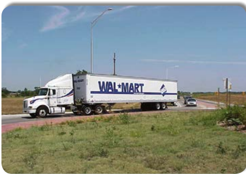
Figure 3: Truck navigating a roundabout Source: KDOT
