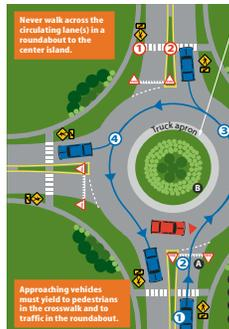
This diagram of a single-lane roundabout is an example only and does not represent all roundabout designs.
