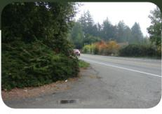
**C2 – Change horizontal and/or vertical alignment of approaches to provide more sight distance**
