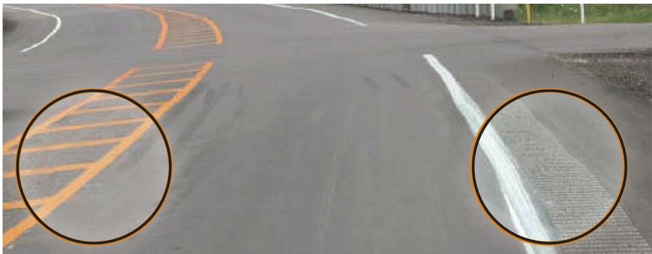
Figure 6: Lane Narrowing Using Rumble Strips
