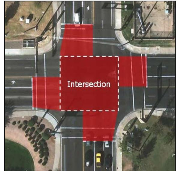
**Figure 1: Diagram of UVC definition of an intersection**
