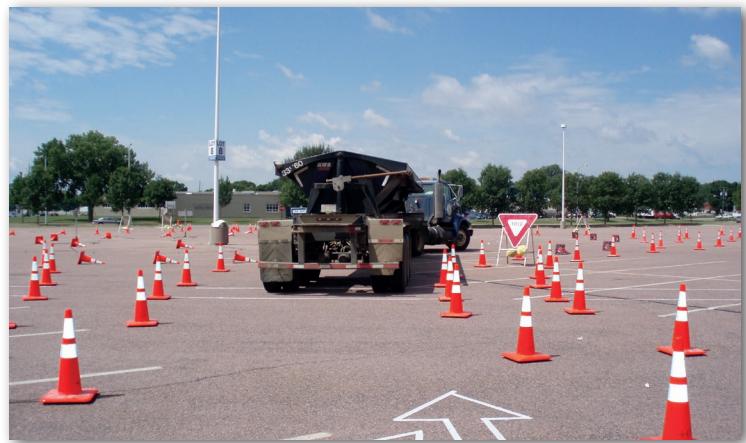
Figure 4: A view of Sioux Falls' mock driveable roundabout set up in a nearby parking lot.
