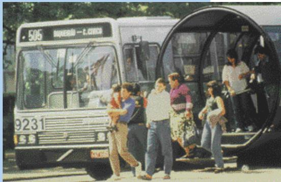
*Bus rapid transit offers many of the features of a subway system—unimpeded vehicle movements, efficient fare collection, quick loading, and reliable service—but above-ground and visible. These advancements are possible through the use of dedicated bus lanes or bus streets; engineering improvements such as bus turnouts and traffic signal preference and preemption at intersections; and enclosed bus-level boarding areas that allow passengers to pay fares prior to entering the bus.*
