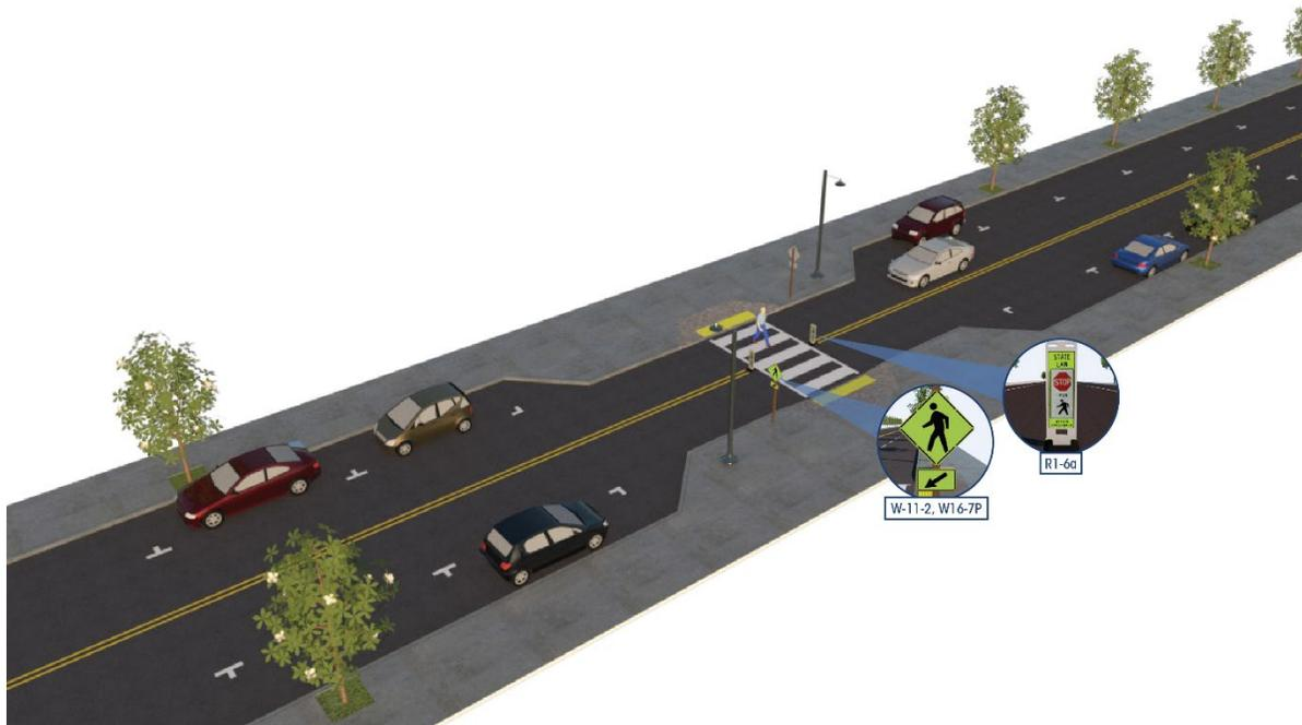
Figure 30. Graphic. Concept featuring pedestrian warning and regulatory signs (W11-2, W16-7PL, and R1-6A) (FHWA, 2018e).
