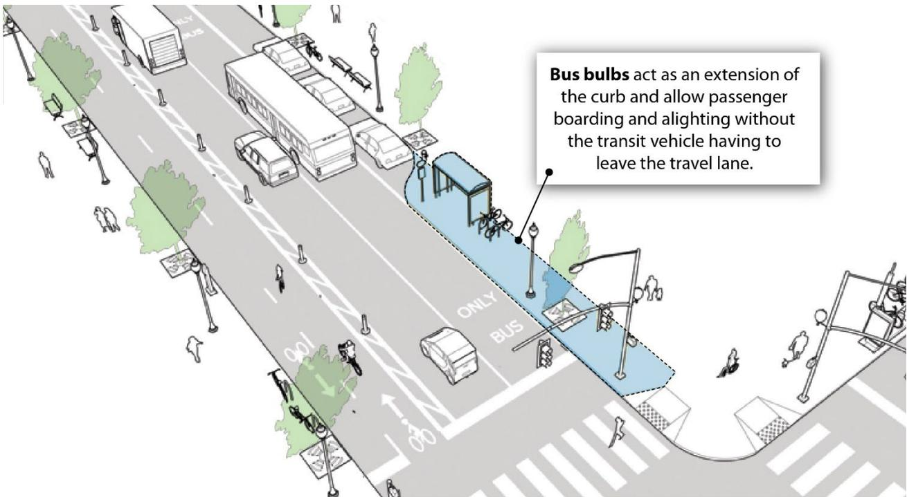
**Bus bulbs** act as an extension of the curb and allow passenger boarding and alighting without the transit vehicle having to leave the travel lane.
