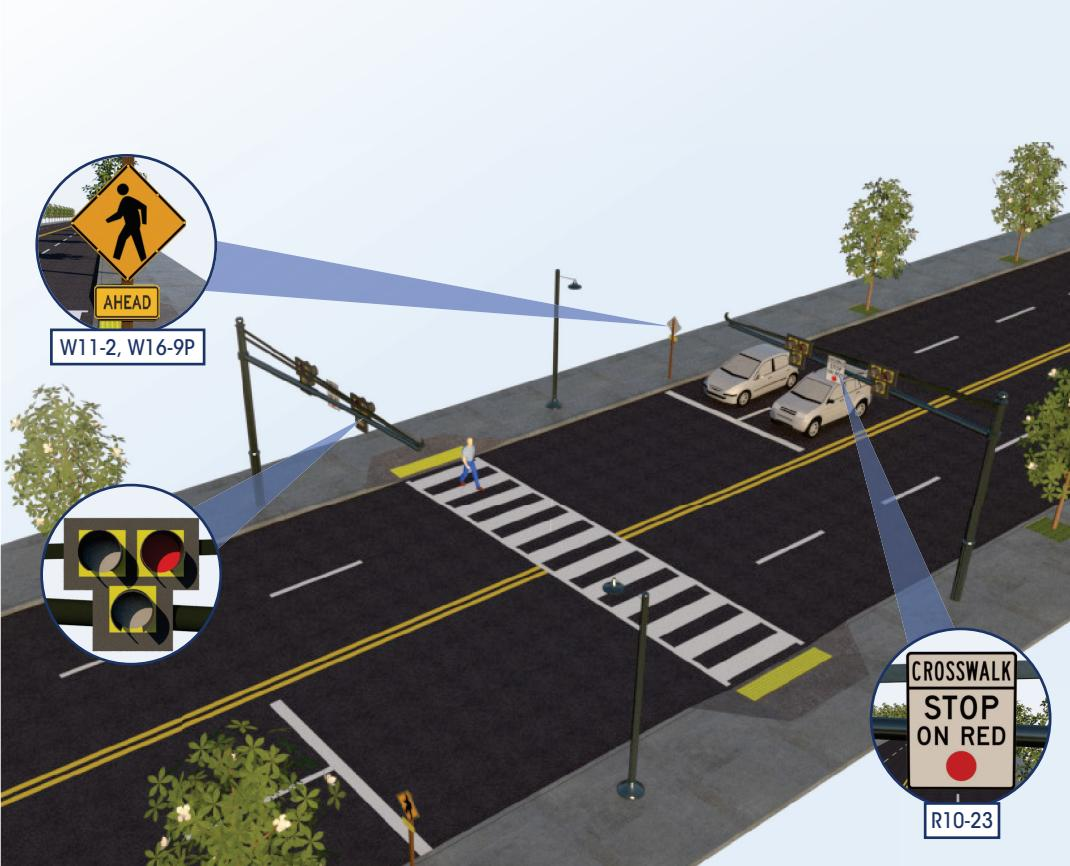
A Pedestrian Hybrid Beacon head consists of two red lenses above a single yellow lens. Unlike a traffic signal, the PHB rests in dark until a pedestrian activates it via pushbutton or other form of detection. When activated, the beacon displays a sequence of flashing and solid lights that indicate the pedestrian walk interval and when it is safe for drivers to proceed (see figure on back page).
