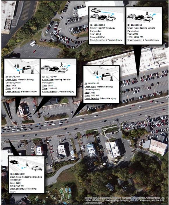
©2019 VHB. Figure 28. Graphic. Collision diagram with pedestrian crash details.
