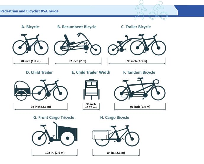
Source: 2020 FHWA. Figure 16. Graphic. Variation in bicycle dimensions. Adapted from FHWA.<sup>(31)</sup>
