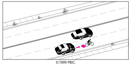
Figure 4. Graphic. Motorist overtaking crash type.<sup>(11)</sup>
