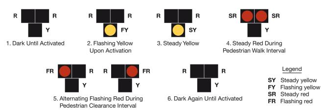
Figure 3. Corresponding Display Sequence for PHB and Pedestrian Signal
