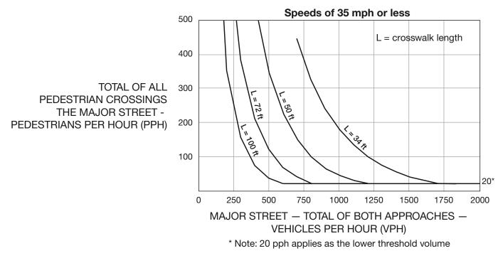
Figure 4. MUTCD Figure that shows recommended thresholds for consideration of PHBs
