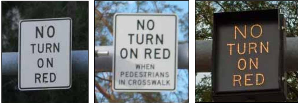
**Figure 13. Static and Active NTOR Signs Tested in Miami**
