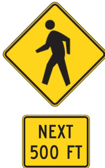
**Figure 12. MUTCD W11-2 Pedestrian Warning Sign and Supplemental Distance Plaque**
