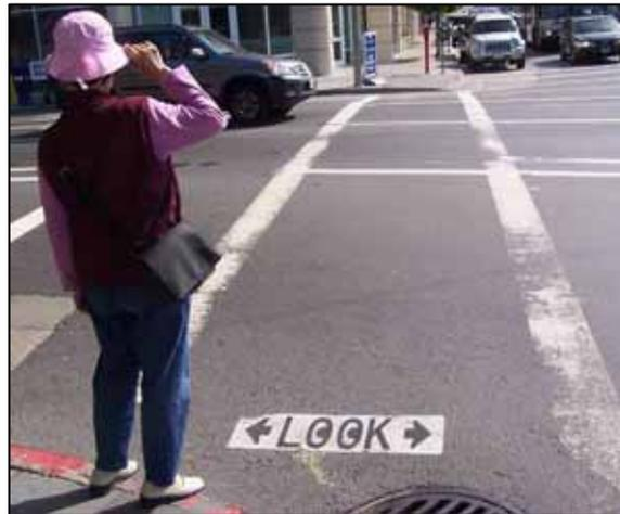
**Figure 21. LOOK Pavement Stencils Tested in San Francisco**
