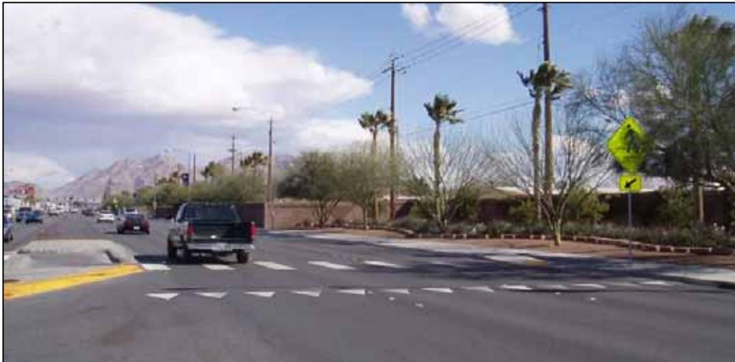
**Figure 41. Advanced Yield Markings installed at Lake Mead Boulevard: Belmont Street to McCarran Street**
