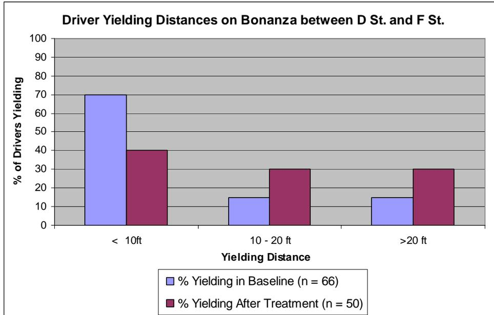
**Figure 11. Yielding Distances at Las Vegas Site Before and After Installation of In-street Pedestrian Signs**
