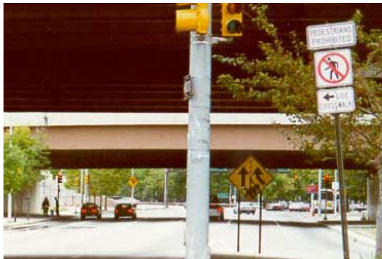
Pedestrians are restricted from continuing straight and are encouraged to cross to the left to avoid a vehicular merge lane.
