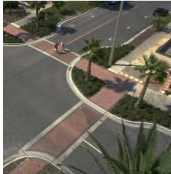
Bulb-outs reduce crossing distances for pedestrians.
