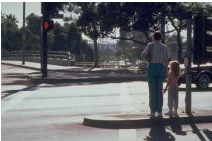
Refuge islands provide a safety area for pedestrians who cannot cross the entire street on one cycle.
