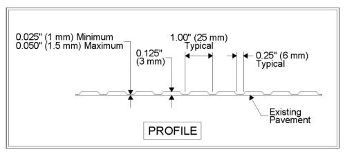
Figure 19a. Illustration. An inverted profile where depressions are made every 1 inch along the stripe.
