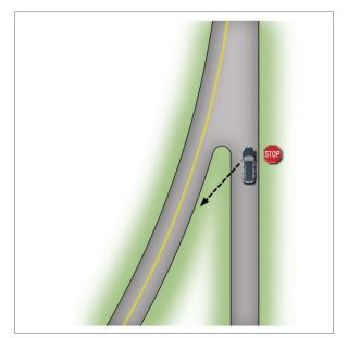
Figure 69. Illustration. Intersection with a skewed approach with an arrow indicating the driver's line of sight.
