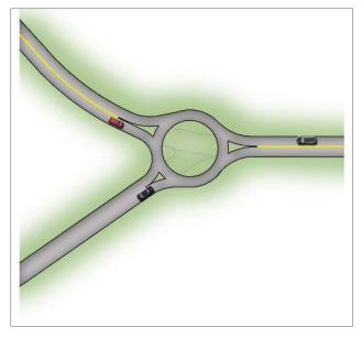
Figure 73. Illustration. Reconfiguring the intersection with a roundabout.
