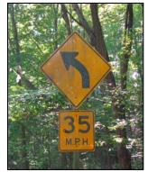
Figure 38. Photo. Low Retroreflectivity sign example.
