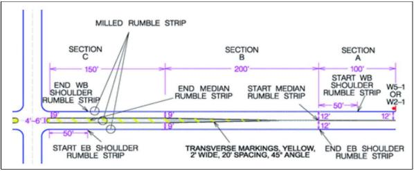
Figure 61. Illustration. Smooth lane narrowing typical design.
