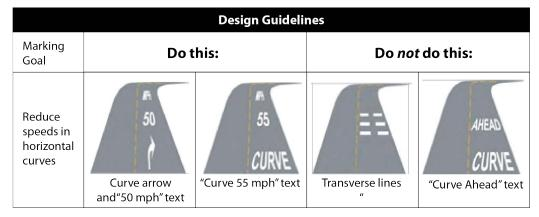
Figure 14. Illustration. Design Guidelines for Pavement Markings to Reduce Speeds at Horizontal Curves. Source: NCHRP Report 600.
