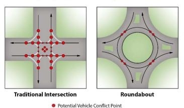
With roundabouts, head-on and high-speed right angle collisions are virtually eliminated.
