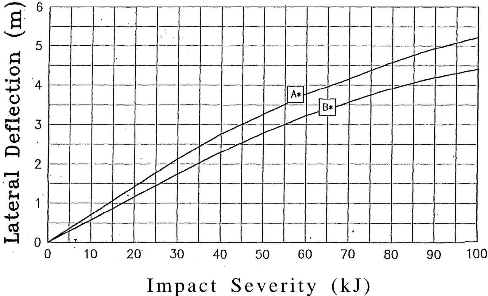
\* Data for curves A and B were obtained from test conducted on installation positioned on a clean asphalt foundation with less than 5% cross slope using 820 to 2000 kg vehicles. When setting up work zones, the expected lateral deflection of the barrier should be accounted for to ensure maximum protection of the workers
