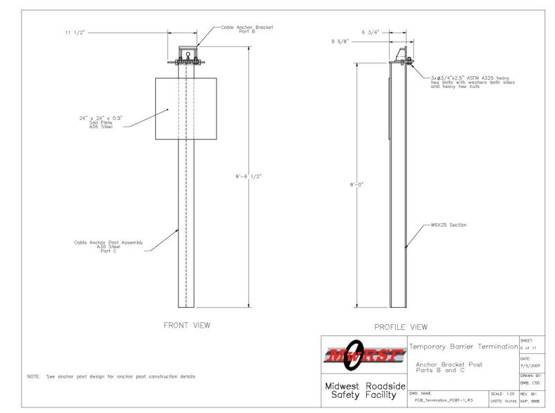
Figure 51. Termination of Temporary Concrete Barrier, Final Design Details
