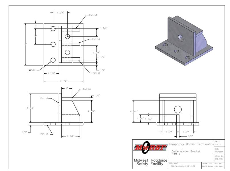
Figure 52. Termination of Temporary Concrete Barrier, Final Design Details
