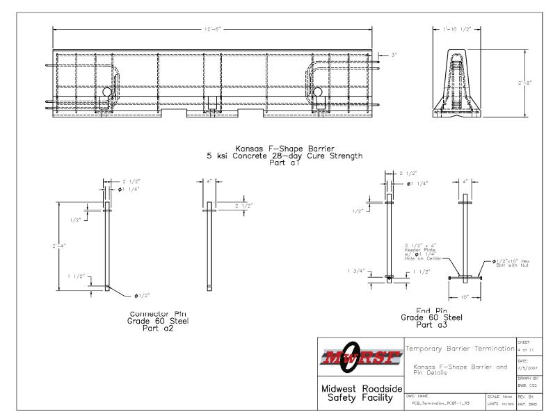
Figure 49. Termination of Temporary Concrete Barrier, Final Design Details
