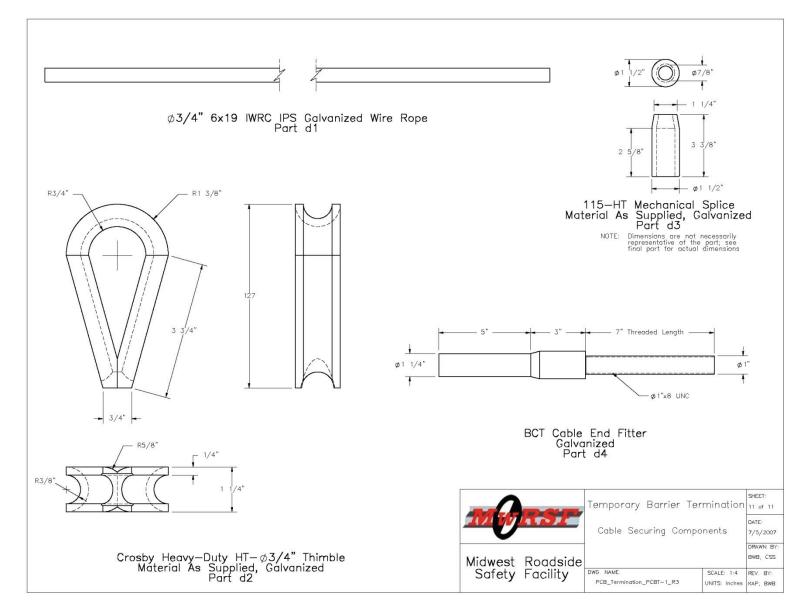
Figure 56. Termination of Temporary Concrete Barrier, Final Design Details
