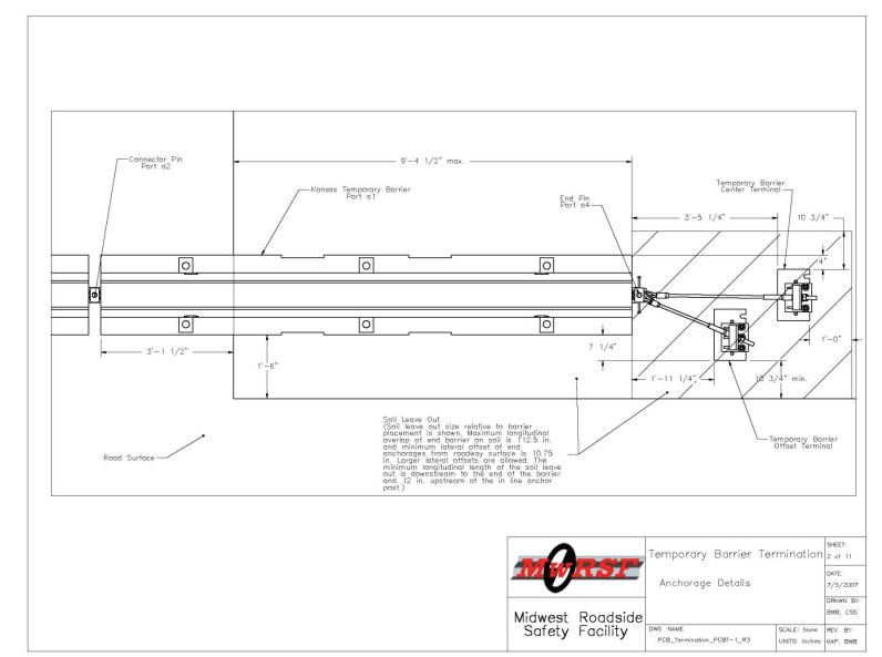
Figure 47. Termination of Temporary Concrete Barrier, Final Design Details
