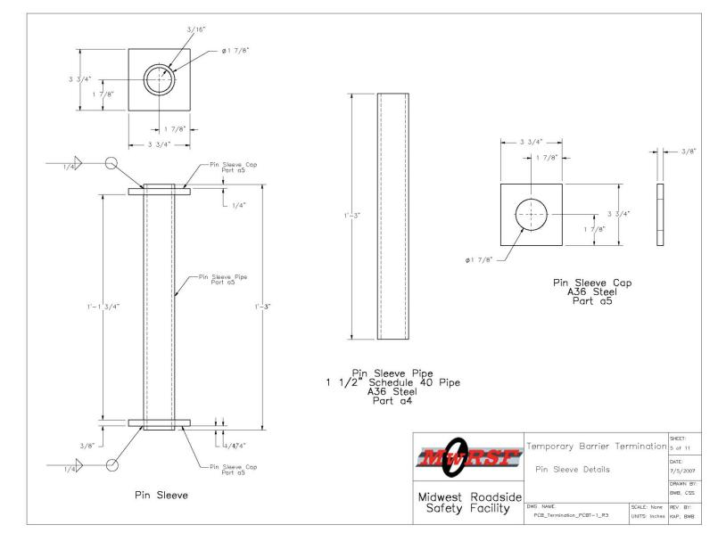
Figure 50. Termination of Temporary Concrete Barrier, Final Design Details
