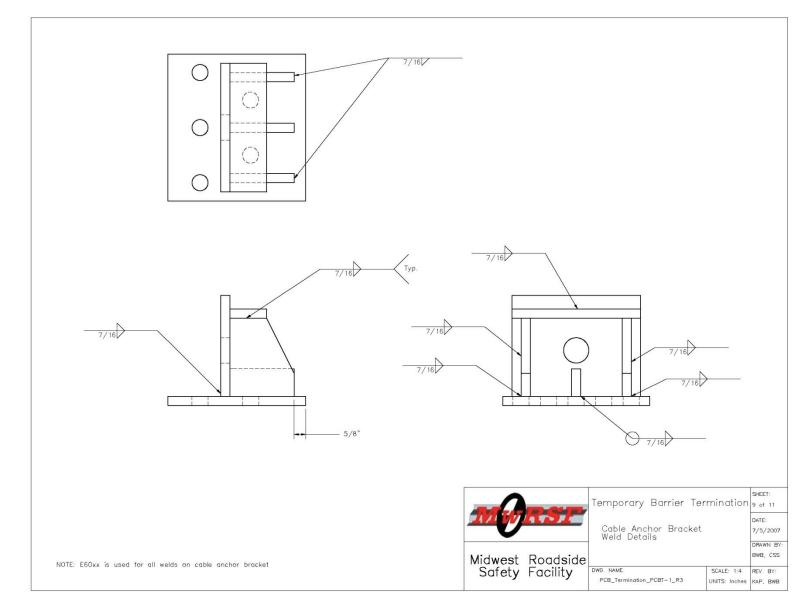
Figure 54. Termination of Temporary Concrete Barrier, Final Design Details
