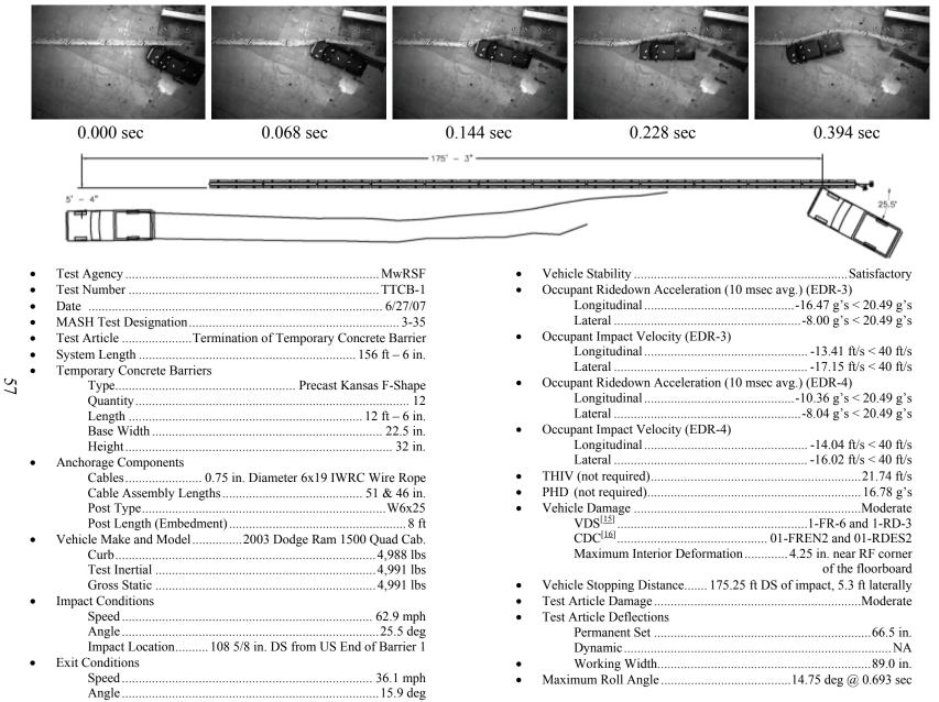
Figure 26. Summary of Test Results and Sequential Photographs, Test No. TTCB-1
