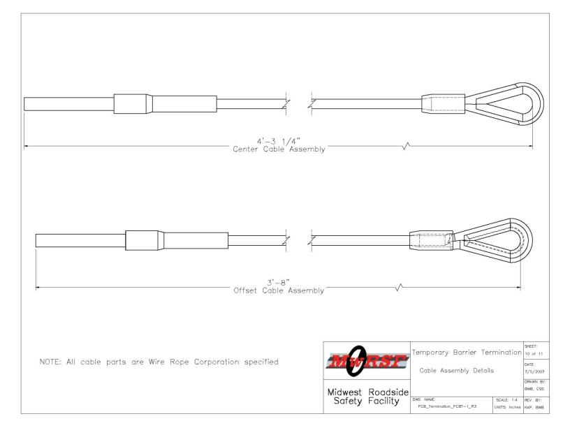
Figure 55. Termination of Temporary Concrete Barrier, Final Design Details
