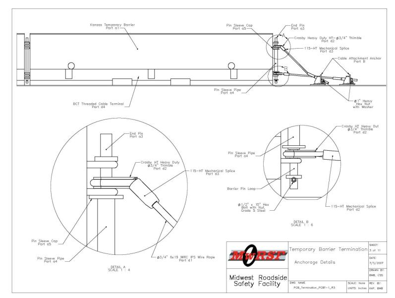
Figure 48. Termination of Temporary Concrete Barrier, Final Design Details
