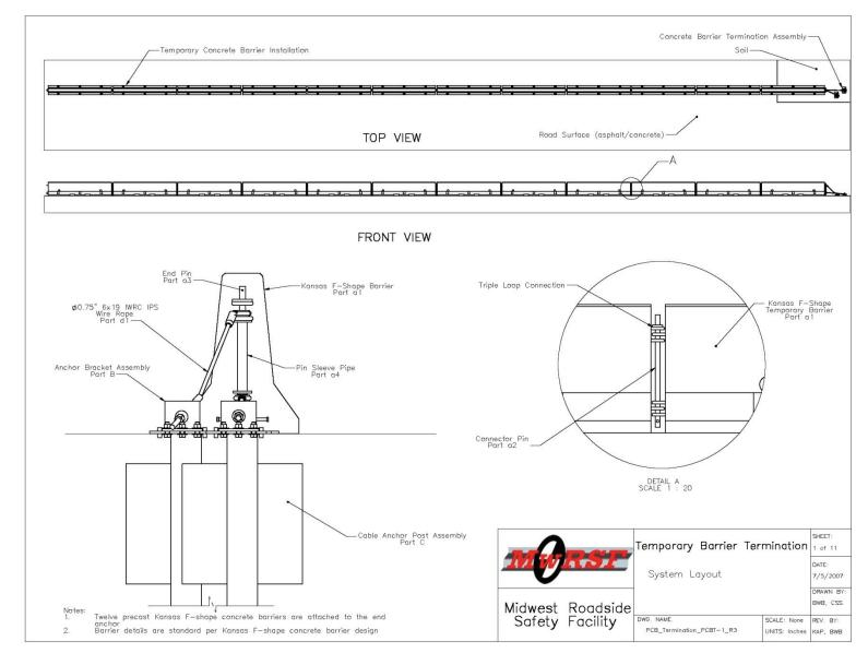
Figure 46. Termination of Temporary Concrete Barrier, Final Design Details
