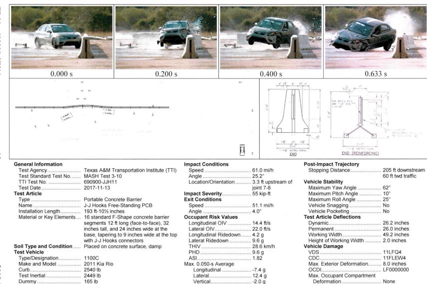
Figure 5.7. Summary of Results for MASH Test 3-10 on J-J Hooks® Free-Standing PCB.
