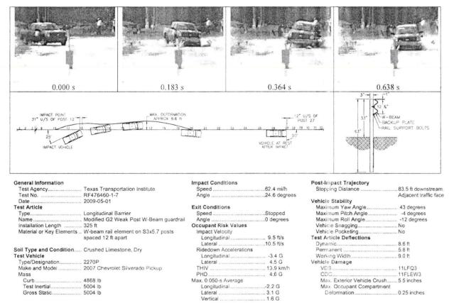
Figure 81. Summary of Results for MASH Test 3-11 on the Modified G2 Weak Post W-Beam Guardrail.
