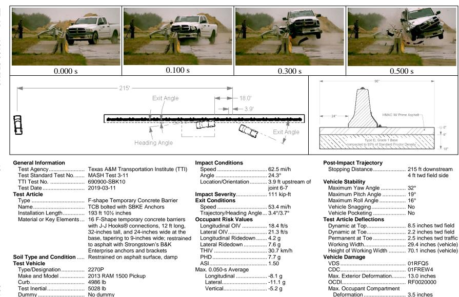
Figure 5.6. Summary of Results for *MASH* Test 3-11 on Temporary Concrete Barrier with SBKE Anchors and Brackets Anchored to Asphalt.
