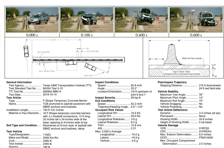
Figure 5.6. Summary of Results for *MASH* Test 3-10 on TCB Anchored to Asphalt Pavement with SBKE Anchors and Brackets.
