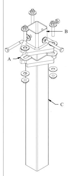
Complete Slip Base Assembly for Concrete Installation
