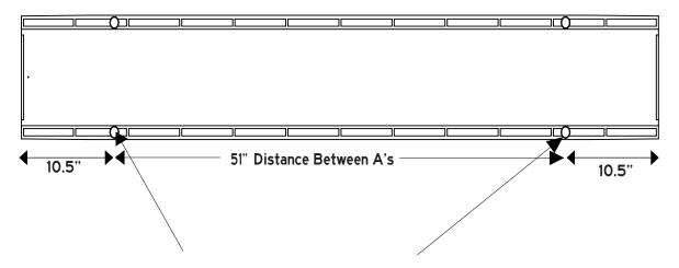
The circles in this drawing represent a "stop" to keep the A's in a fixed position
