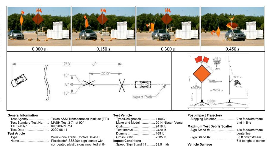
Figure 6.7. Summary of Results for *MASH* Test 3-71 at 90 Degrees on Plasticade® SS620A Sign Stands with Corrugated Plastic Signs Mounted at 84 inches.
