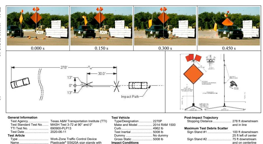
Figure 5.6. Summary of Results for *MASH* Test 3-72 at 0° and 90° on Plasticade® SS620A Sign Stands with Corrugated Plastic Signs Mounted at 84 inches.
