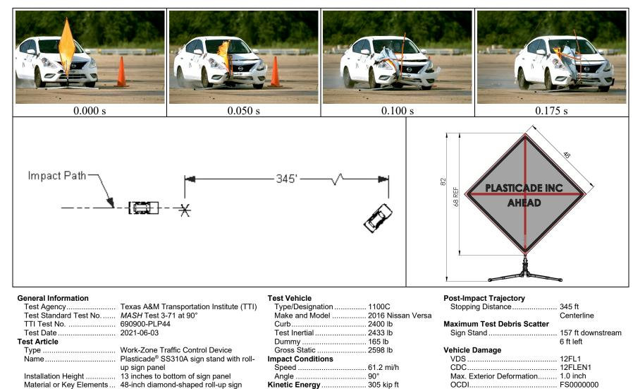
Figure 7.6. Summary of Results for MASH Test 3-71 at 90 Degrees on Plasticade® SS310A Sign Stand with Roll-Up Sign Panel.
