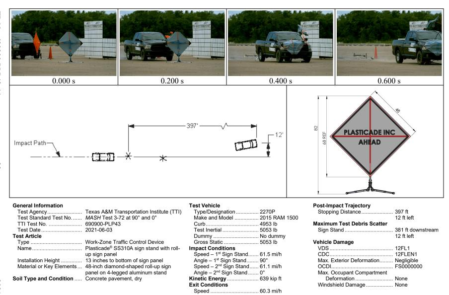
Figure 6.5. Summary of Results for *MASH* Test 3-72 at 90 Degrees and 0 degrees on Plasticade® SS310A Sign Stand with Roll-Up Sign Panel.
