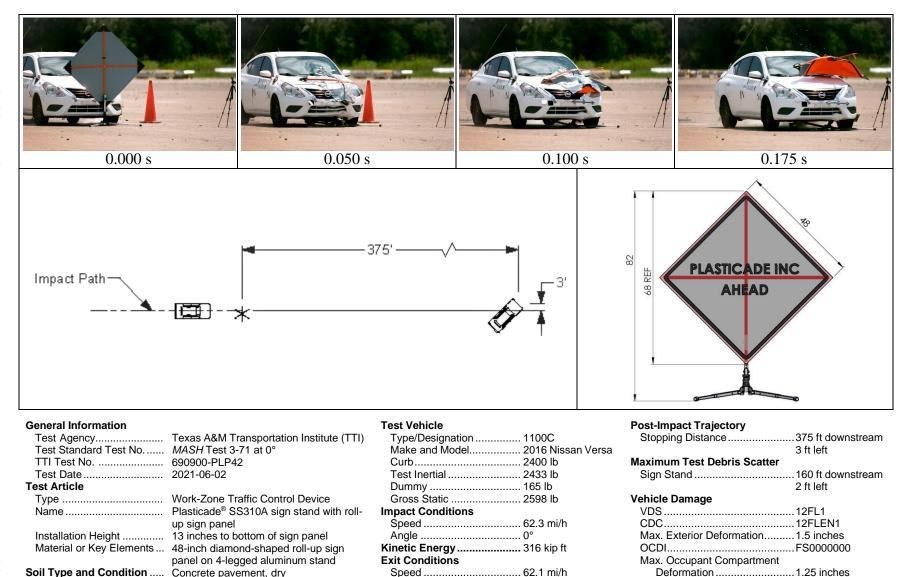
Figure 5.6. Summary of Results for MASH Test 3-71 at 0 Degree on Plasticade® SS310A Sign Stand with Roll-Up Sign Panel.
