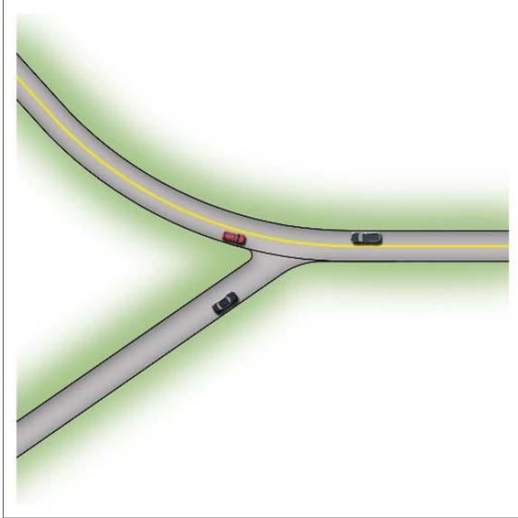
**Figure 71. Illustration. Typical skewed intersection within a curve.**
