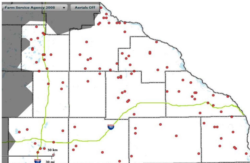
**Figure 3. Map. Severe (K and A) roadway departure crashes at curves over a five year period in Minnesota's southeastern District. The wide dispersion of crashes indicates that a traditional site analysis/spot location approach will not sufficiently address this type of severe crash.**
