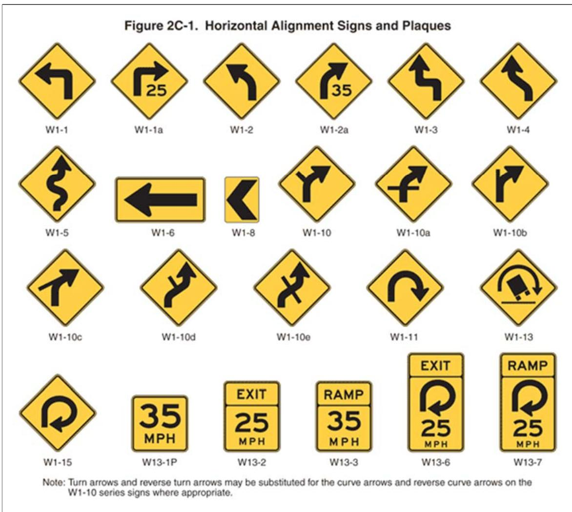
**Figure 20. Illustration. Figure 2C-1 from the MUTCD.**
