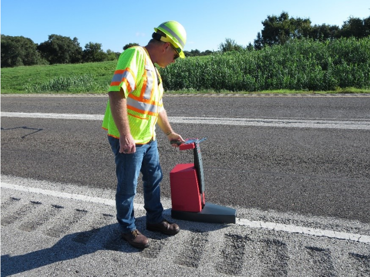
Figure 3. Photo. Measuring retroreflectivity with a handheld instrument.
