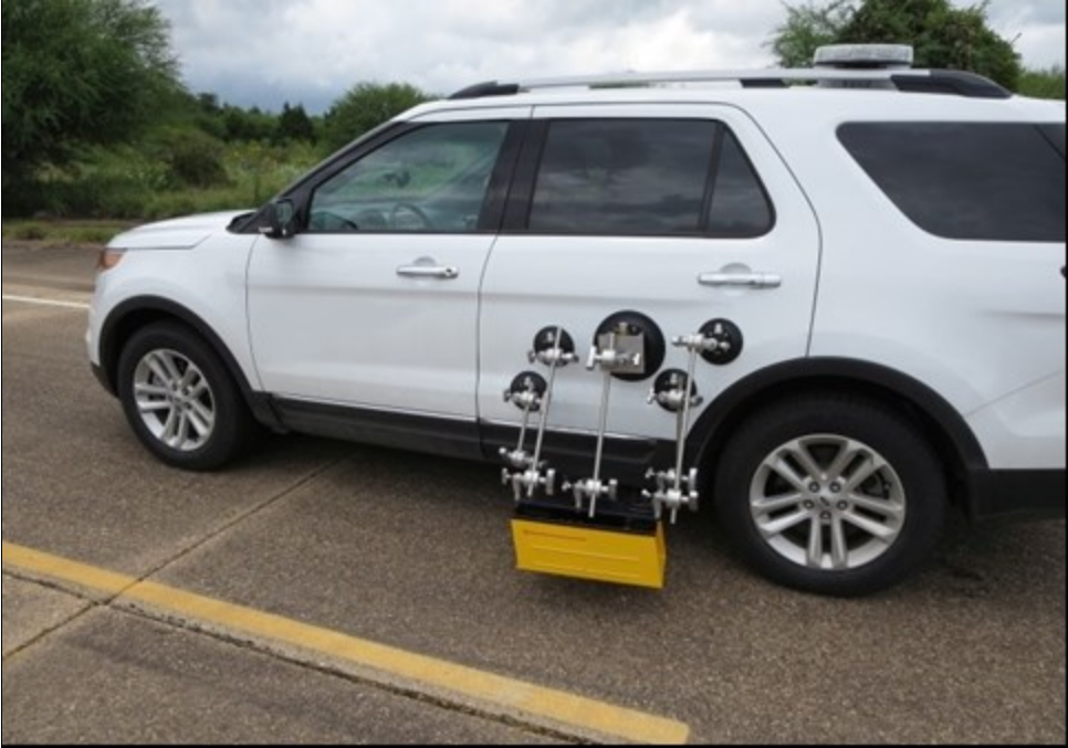
Figure 4. Photo. Typical mobile pavement marking retroreflectivity measurement instrument.
