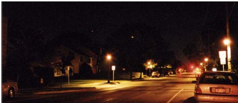
Figure 20 – Example of High Glare Street Lighting
