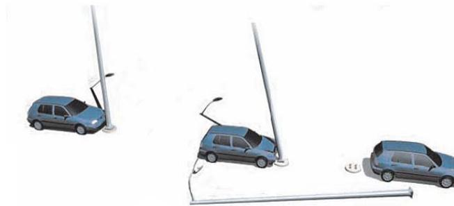
Figure 39 – Pole with Breakaway Device
