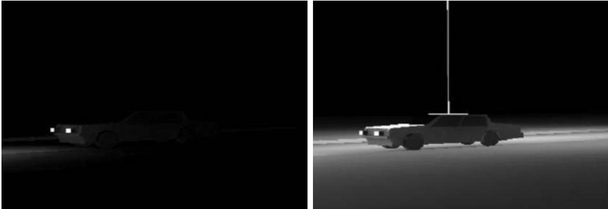
*In the panel to the left, the roadway is lighted only by car headlights. In the panel on the right, the roadway is lighted by car headlights and fixed roadway lighting.*
