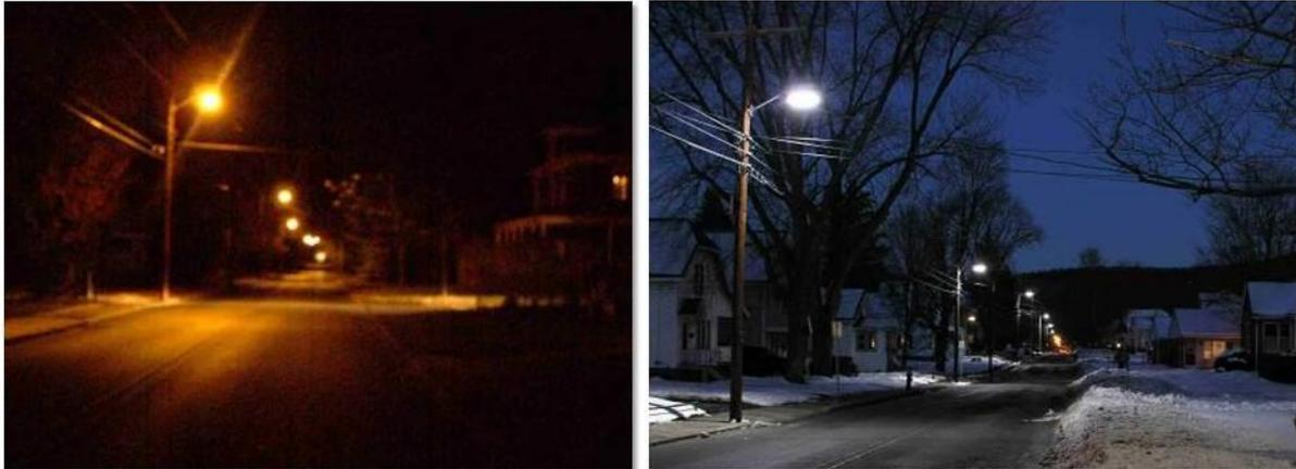
*A street lighted with high pressure sodium (HPS) light sources (left). A street lighted with a “whiter” light source was rated as safer by drivers and pedestrians (right).*
