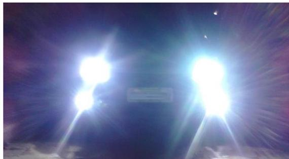
*The vehicle headlamps in this photograph are causing disability glare, significantly reducing visibility for any oncoming drivers.*
