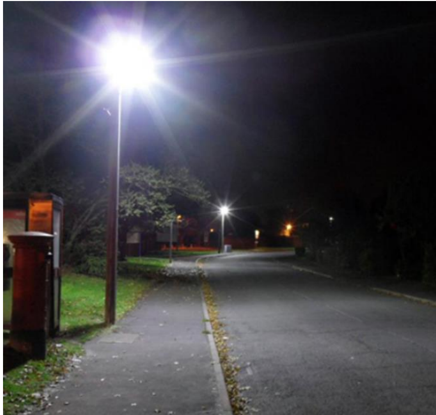
A glaring luminaire along a roadway at night. Lighting engineers use the veiling luminance metric to limit potential glare from roadway luminaires.
