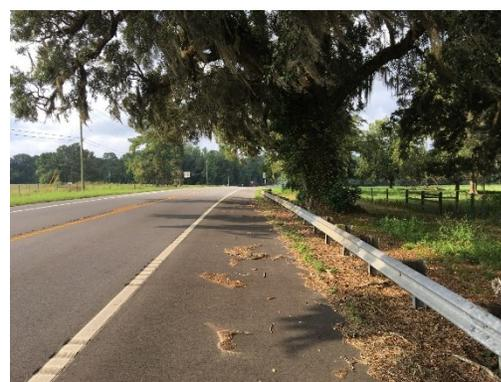
Guardrail shielding large tree. Source: FHWA
