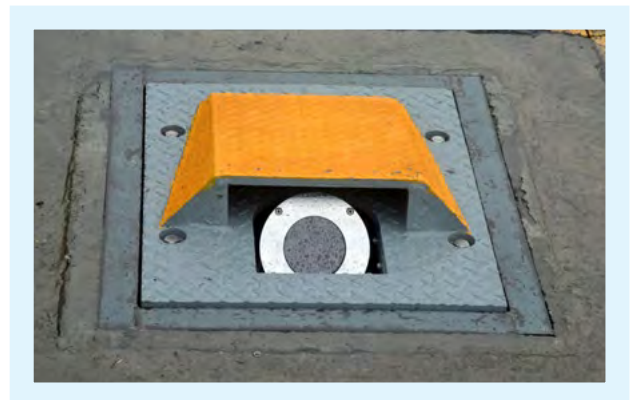
View of camera when placed in roadway. This unorthodox location exposes a perfect view of each brake as the vehicle passes over the camera.
