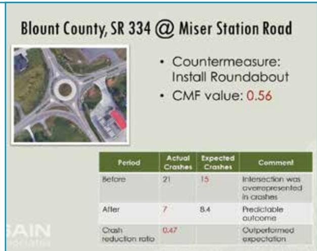
Crash-modification factor analysis of roundabout installation.
