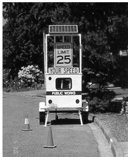
Figure 5.39. Radar Speed Trailer in the Field. (Kirkland, WA)
