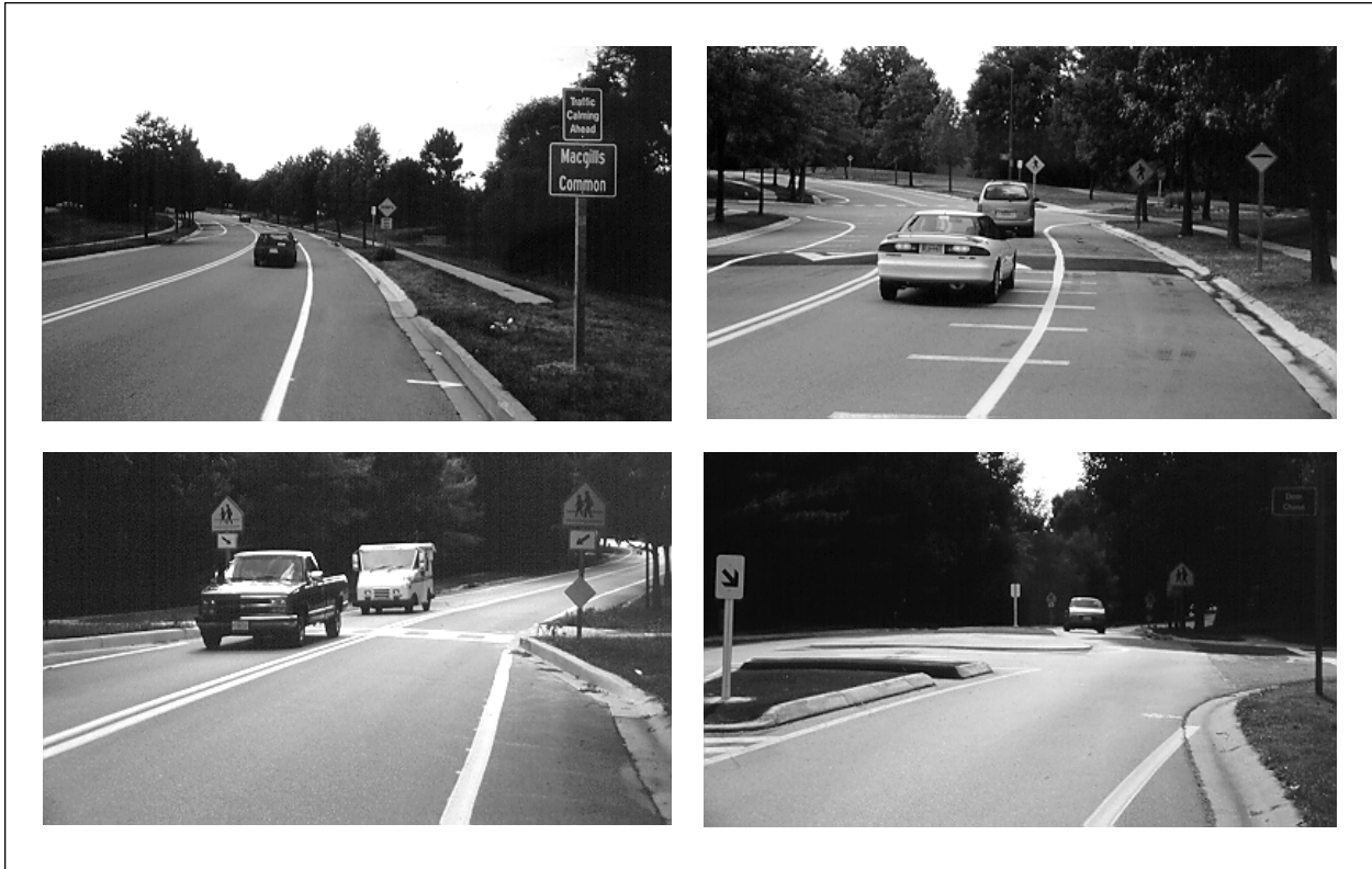
Figure 9.12. Series of Calming Measures on a Major Collector. (Columbia, MD)
