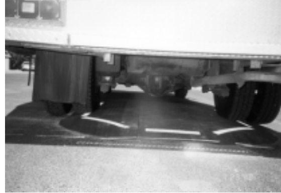
Figure 7.19. Test of a Speed Cushion. (Austin, TX)
