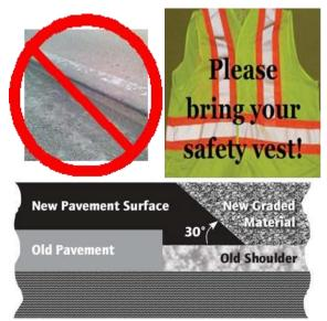
At minimal additional cost, the Safety Edge provides a roadway edge that allows errant vehicles to return to the roadway safely. A stronger transition with the graded material can also reduce the level of maintenance required.
