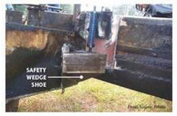
The Safety Edge is created by a shoe installed on the paver to create a 30-degree consolidated wedge.
