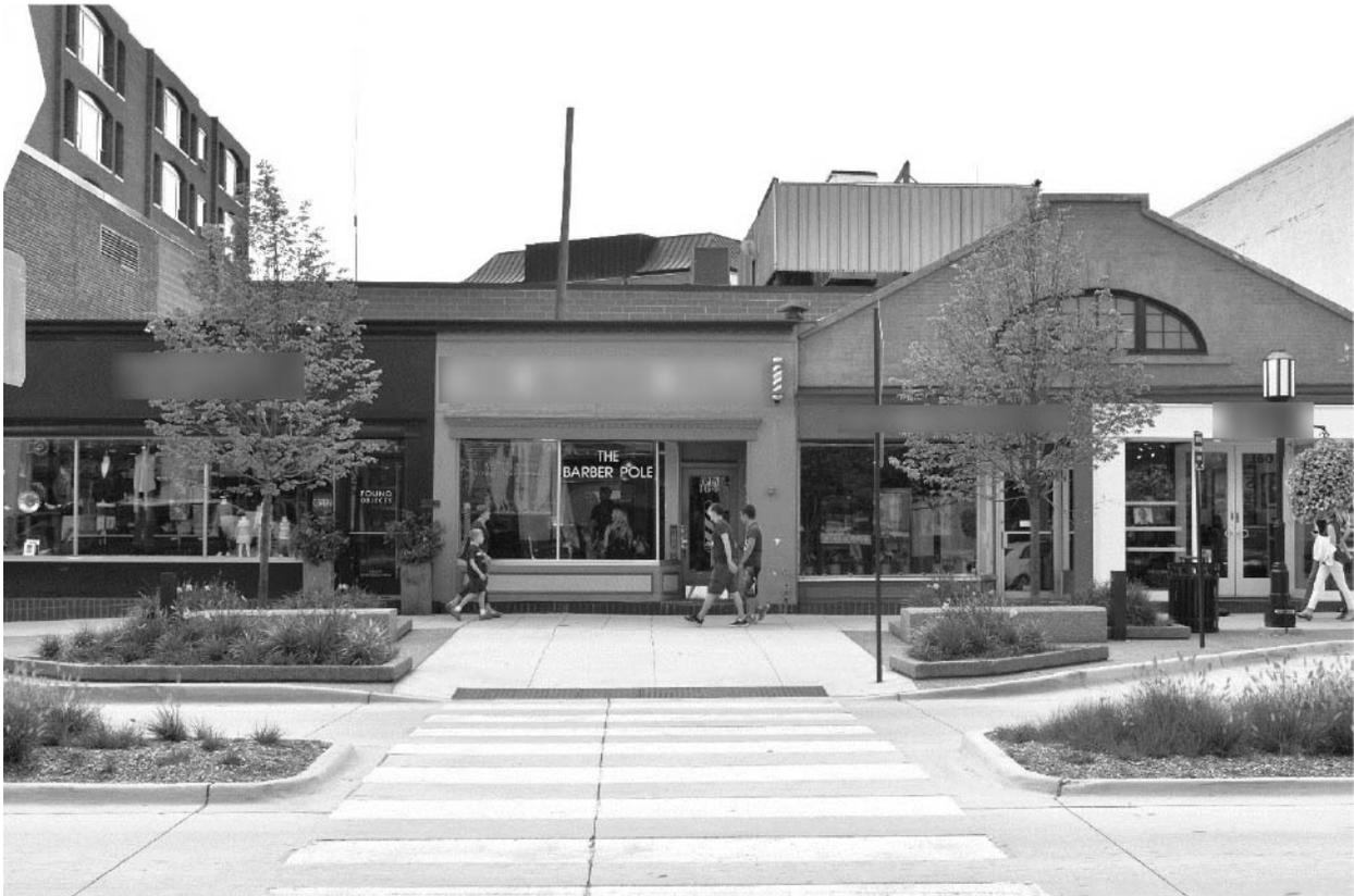
**Figure 4. Redundancy is key—such as high-visibility crosswalks and bumpouts—in a Safe System application to prevent crashes. Source: Mariah Hewines/Unsplash.**
